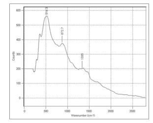
Figure 8: Raman shifts of carbopol934
