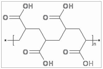
Figure 2: Structure of carbopol polymer (polyacrylic acid)
